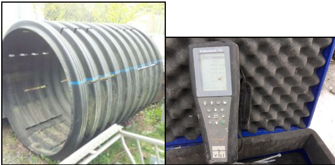
Figure 3: Task 1 Overflow – Example of a refuge pipe measuring 1.5m diameter x 2m length and with slots at regular intervals allowing juvenile fish to enter pipe during low-flow in the side channel (Left; Photo source: DFO) and YSI unit used to monitor temperature and DO in these pipes (right).
