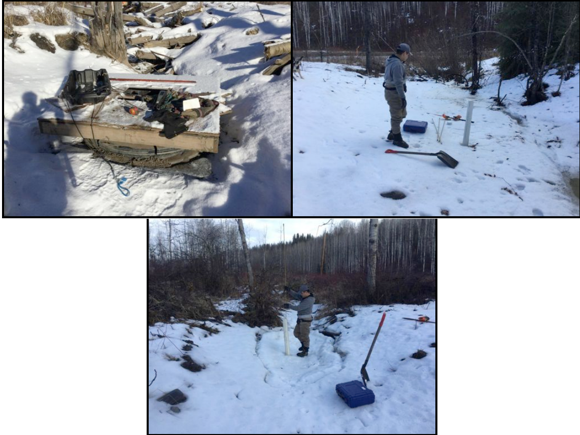
Figure 7: Photo Series showing examples of test and refuge pipe monitoring for groundwater level, temperature and DO in the winter of 2017 (February 14 th and 17 th ). Note the unusually low snow pack in the area.
